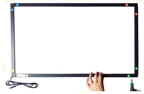
2-5 Turn the product over. There are no labels or stickers. Place the Touch Frame on a flat surface and connect the USB to a computer. We advise testing the product with the computer before mounting it to the monitor.
